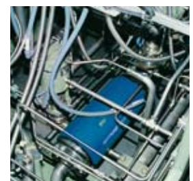
KRAL Volumeter installed in the engine room of a yacht.
