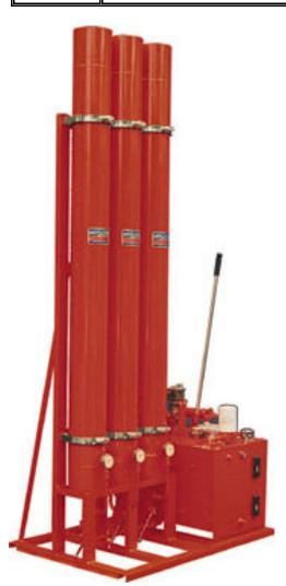
EPS starting system (Variation B) with all components mounted on a frame. 3 accumulators per system, each with a shut off valve and a pressure gauge. The complete system is painted according to the requirement of the customer.
